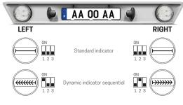
Assembly with 2 rear lamps side by side
